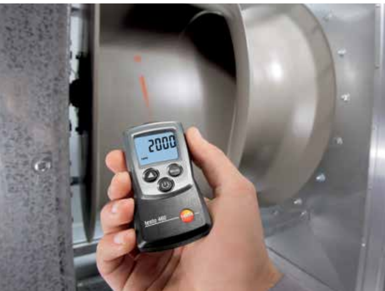
Non-contact measurements on ventilators are possible for example with the handy testo 460. The measurement spot is displayed by an LED marking on the measurement object.
