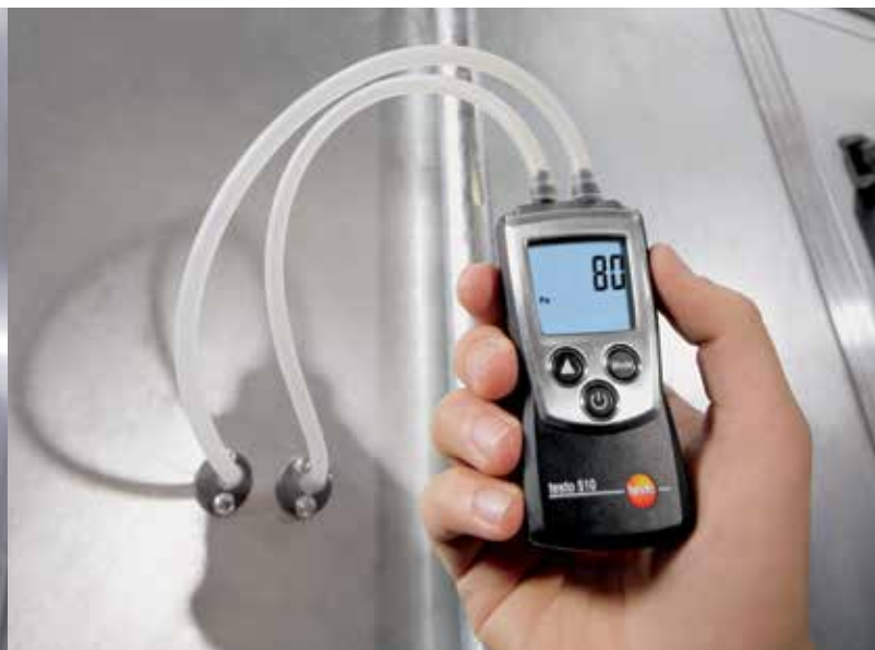
You can quickly and reliably check whether a filter is dirty using the differential pressure measuring instruments from Testo, e.g. the testo 510.
